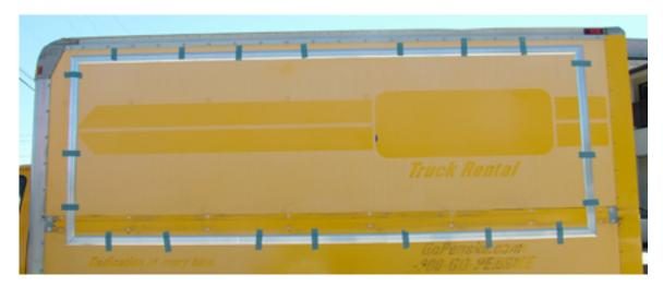
**Temporarily tape the four base plate sides into position using 6 inch duct tape holding tabs.** Tip: Start with the top side section(s) (that's the side with the pencil guide) then do the sides (keeping right angles to the top) and then the bottom. The temporary duct tape holding tabs make it easy to readjust and place all sections into the proper square 90-degree positions before screwing to the truck or wall. See photo above.
